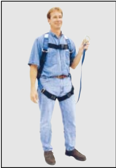
Web Lanyard w/ Safety Harness is Required for Construction by OSHA (effective January 1, 1998 Body Belts not acceptable)
